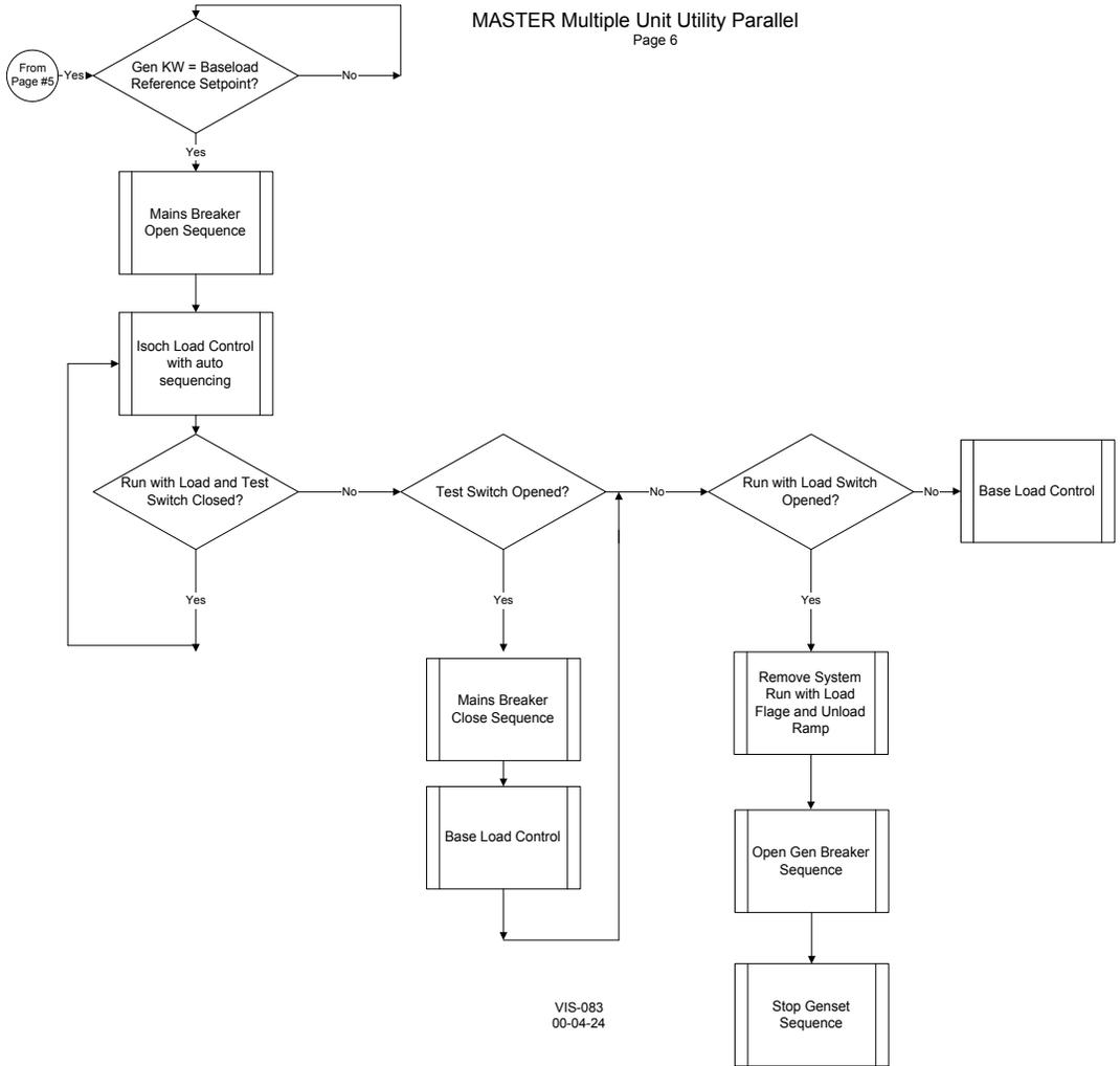
Figure 7-4f. Master Multiple Parallel Process Control Flow Diagram
